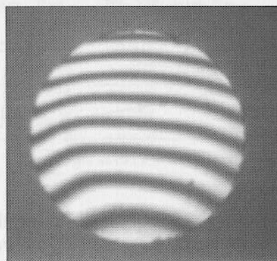
Fig. 9.8 Interferogram of a "flat" mirror.
