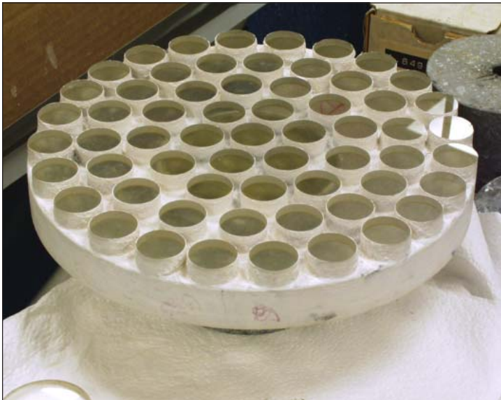
Figure 1 Round optics are easier and more economical to manufacture.
