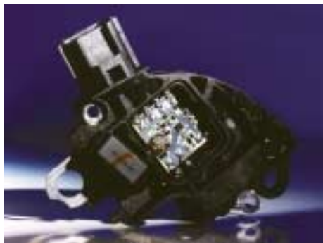
Ceramic circuit with laser beam soldered contacts
