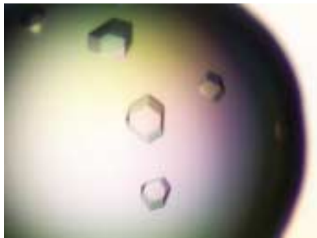
Protein crystal (glucose isomerase) for x-ray diffractometry
