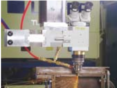
Diode laser cutting of 0,5 mm thick stainless steel
