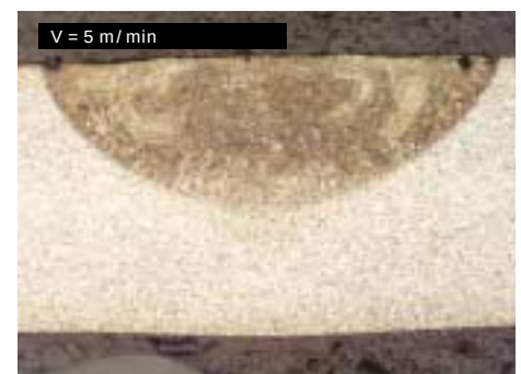
Fig. 1 and 2 from above: Weld seams in 6 mm AlMg- alloy, v = 150 \text{ mm/min} . Fig. 3 and 4: Weld seams in 2 mm AlMg-alloy with graphik layer.
