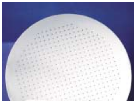
Fig.1: Embossing tool in \text{Al}_2\text{O}_3 Fig.2: Laser drilled holes in sapphire wafer Fig.3: Hollowed out silicon structure
