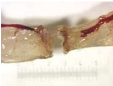
Above: Laser anastomosis of spermatic duct (rat model) Below: Test sample following tensile strength test
