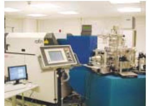
Prototype of the MOPA system with connected EUV-plasma-chamber (photo: Xtreme technologies)
