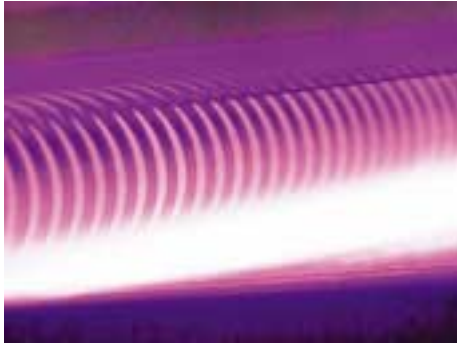
Atmospheric-pressure plasma produced by a dielectric barrier discharge
