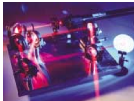
Mach-Zehnder interferometer to study the interaction of laser pulses with nanolitre droplets
