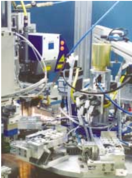
laser drilling machine to remove the middle pole of halogen capsules
