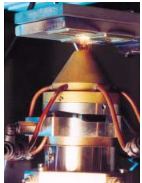
Above: Mobile 5-axis-system (Schuler Held Lasertechnik) Below: Overhead cladding with the three-way nozzle with integrated cross jet
