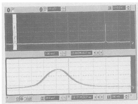
Fig. 5. The frequency fluctuation ( \pm 220 kHz) in 1 minute under the condition of laser running with frequency-stabilizing system on but without temperature controlling of F-P2.
