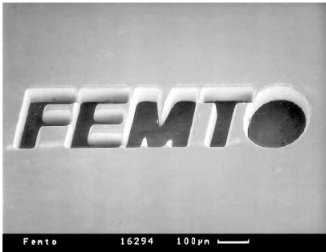
Fig. 5. Example for microstructuring of metals by femtosecond pulses: ablation of tungsten by amplified femtosecond Ti:sapphire pulses of pulse duration \tau_p \approx 100 fs, pulse energy E_p \approx 1 mJ at 1-kHz repetition rate at \lambda = 780 nm [135]. Photograph courtesy of S. Nolte and B.N. Chichkov, Laser Zentrum Hannover, Hannover, Germany
