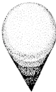
Figure 3.5 The coma patch. The image of a point source is spread out into a comet-shaped flare.
