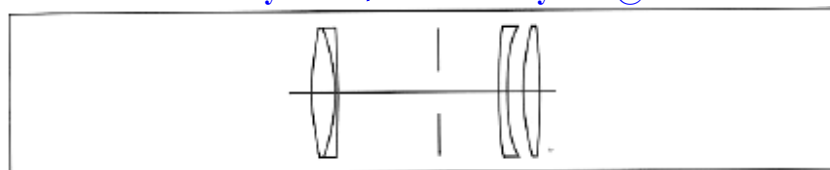
Fig. 33.1 Traditional Petzval lens form.
