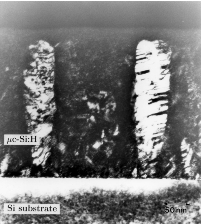
Fig. 1. Dark field transmission electron microscopy micrograph of a \mu\text{c-Si:H} film grown at \text{SC} = 2\% and a plasma excitation frequency of 95 MHz.
