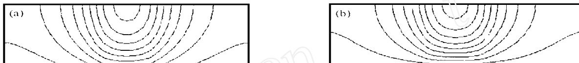
Fig 5 Calculated temperature distribution in slab
