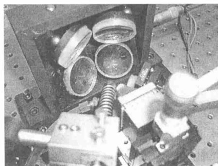
Fig.3 View of the experimental setup of the Yb:YAG thin disk laser
