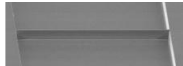
Fig 10. Beam fixed at both ends. The beam is 1mm in length, 100 \mu\text{m} in height, and 50 \mu\text{m} in width.
