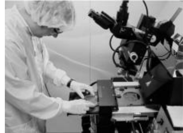
Fig 4. Modified mask aligner for implementing the wafer scale sol-gel on Glass replication process.
