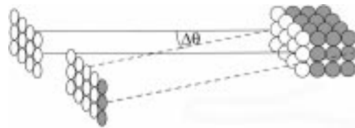
Fig. 11. Two views of a cubic array are formed by parallel projection. The minimum angle ( \Delta\theta ) between the views required for there to be a distinct difference in view content is that required to make one column of rear pixels fully visible.
