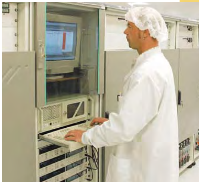
Burn-In: Long-term testing of diode laser elements
