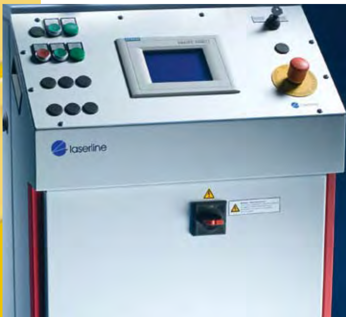
Supply unit with chiller, power supply and integrated laser head
