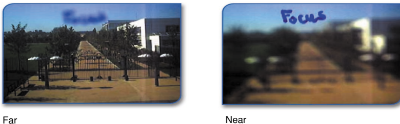
Fig. 1. Light emitted, focused by changing shape of interface
